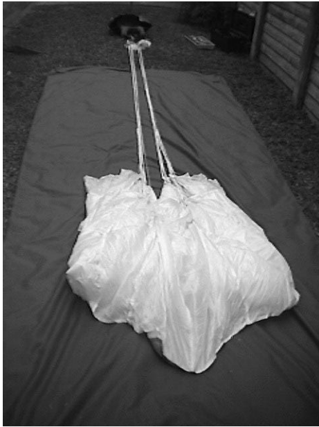
18. Place the B lines on top of the A lines.
