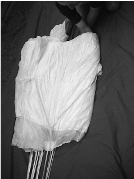
18. Place the B lines on top of the A lines.
